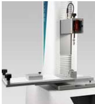
TX-SFF : SLIDING FRICTION FIXTURE (Ref. 120013R)
