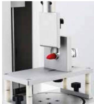
TX-LCF : LIPSTICK CANTILEVER FIXTURE (Ref. 130147R)
