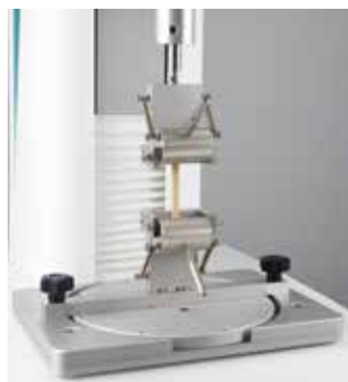
TX-RTF : ROLLER TENSILE FIXTURE (Ref. 130194)
