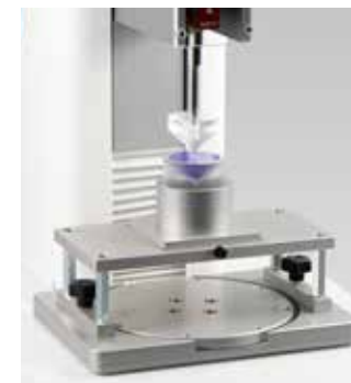
TX-STF : SPREAD TEST FIXTURE (Ref. 130157R)
