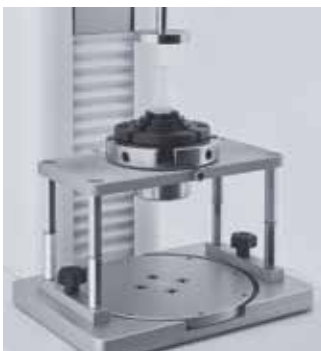
TX-SAF : SYRINGE ACTUATOR FIXTURE (Ref. 130145)
